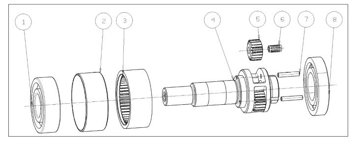
Figure 7: Parts assembly terminal planetary gear system
