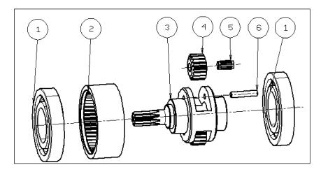
Figure 7: Parts assembly intermediate planetary gear system
