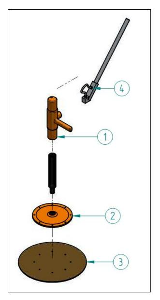
Fig. 2: Parts pneumatic power trowel LAP 45
