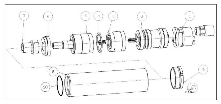
Figure 3: Parts pneumatic motor LAP 45
