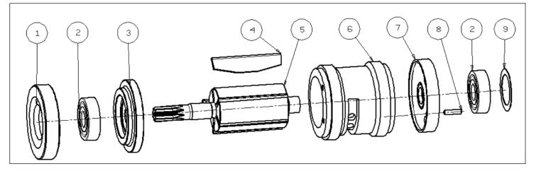
Figure 5: Parts of pneumatic air motor LAP 45
